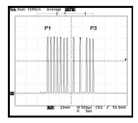
Figure 3-4. Altitude-Coded Pulses
